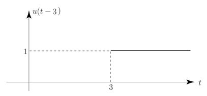
The step function has a useful property: multiplying an ordinary function f(t) by the step function u(t) changes it into a causal function; e.g. if  $f(t) = \sin t$  then  $\sin t \cdot u(t)$  is causal.
